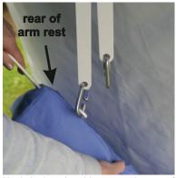
Hook the long (rear) hanger to the rear of the arm rest and the short (front) hanger to the front of the arm rest. Make sure the quick links are tightened after.
