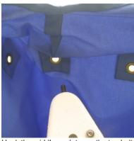
Hook the middle eyelet over the top bolt. The other eyelets are used to adust the awning back and forwards.
